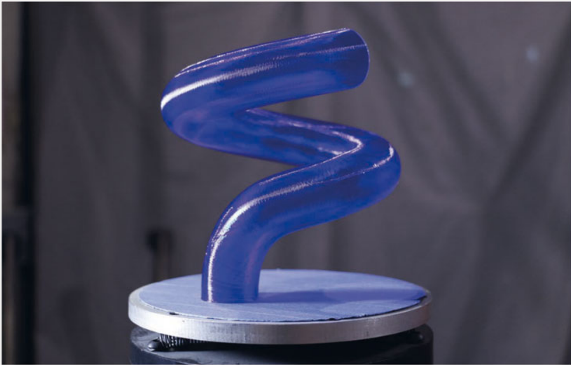
Figure 5: Helical pipes printed in mid-air
